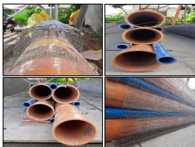
Fig. 4: Orientation of 1/2" uPVC blue pipes and 8mm Ø bars
